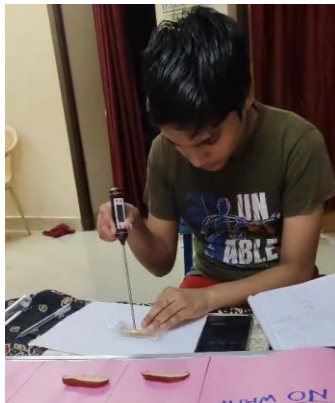
Fig 1(d): Measuring the temperature of apples wrapped in TGB film using a kitchen thermometer.
