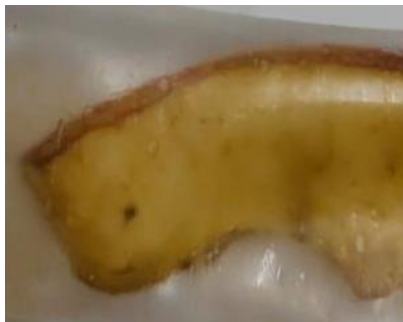
Day 5 — Plain Film (Starch + TSP) visible shrinkage due to water loss.
