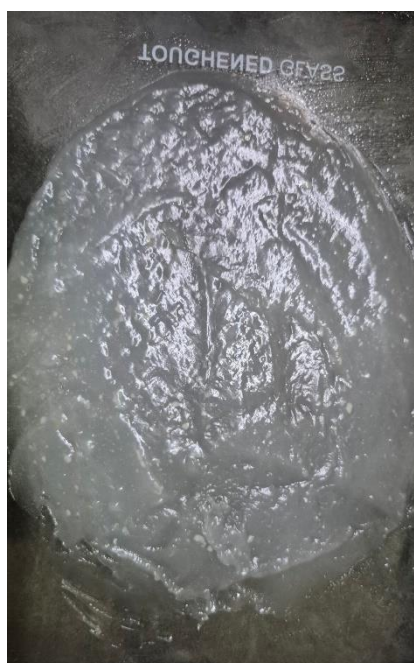
Fig. 3(g): Freshly poured film for drying.
