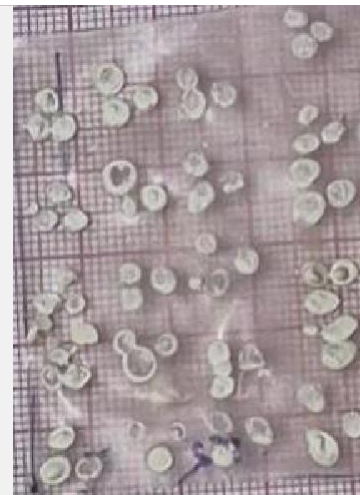
Fig.5 (b): Film with 3 dots/cm 2 – light pattern, clear surface.
