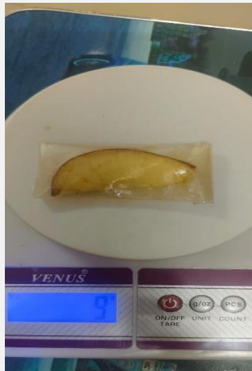
Fig 6(e): Plain starch film weight-loss check: digital balance reading for apple wrapped in base starch film
