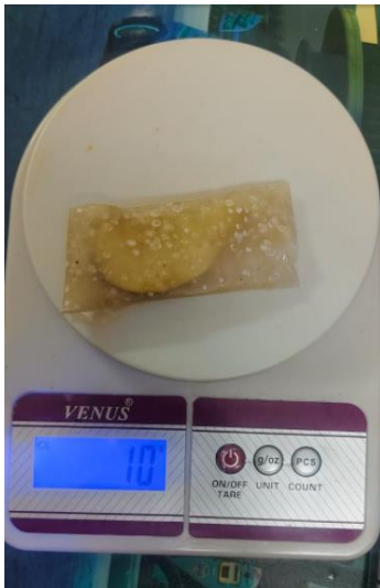
Fig 6(d): TGB film Weight loss check: digital balance reading or apple wrapped in TGB film
