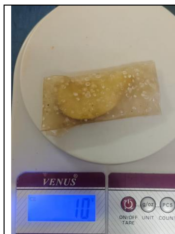
Fig. 5(d): Apple piece wrapped with the 2-dot film at the start of the weight test
