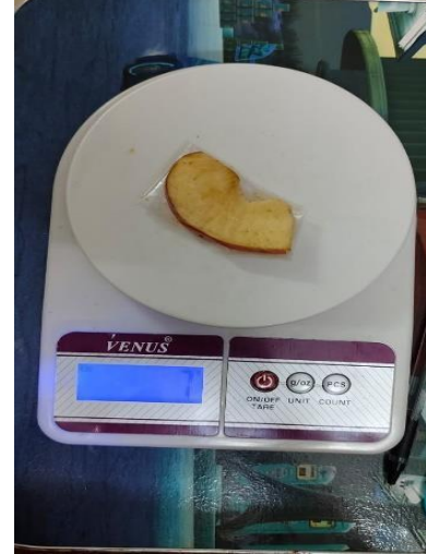
Fig 6(d): Plastic wrapper weight-loss check digital balance reading for apple kept without any wrap
