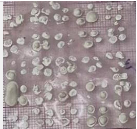
Fig.5(c): Film with 4 dots/cm 2 – Less flexible pattern,
