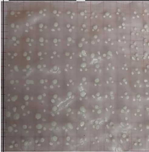
Fig 6(b): TGB film with zeolite and GSE coating: even dot pattern and glossy Finish.
