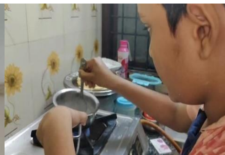
Fig. 3(c): Heating the starch mixture to form the film paste
