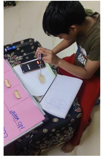
Fig 6(i): Measuring the temperature of apples wrapped in Starch film using a kitchen thermometer
