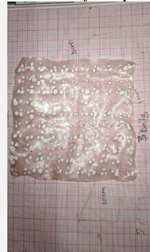
Fig 6(a): TGB film with zeolite and GSE coating: even dot pattern and glossy finish.
