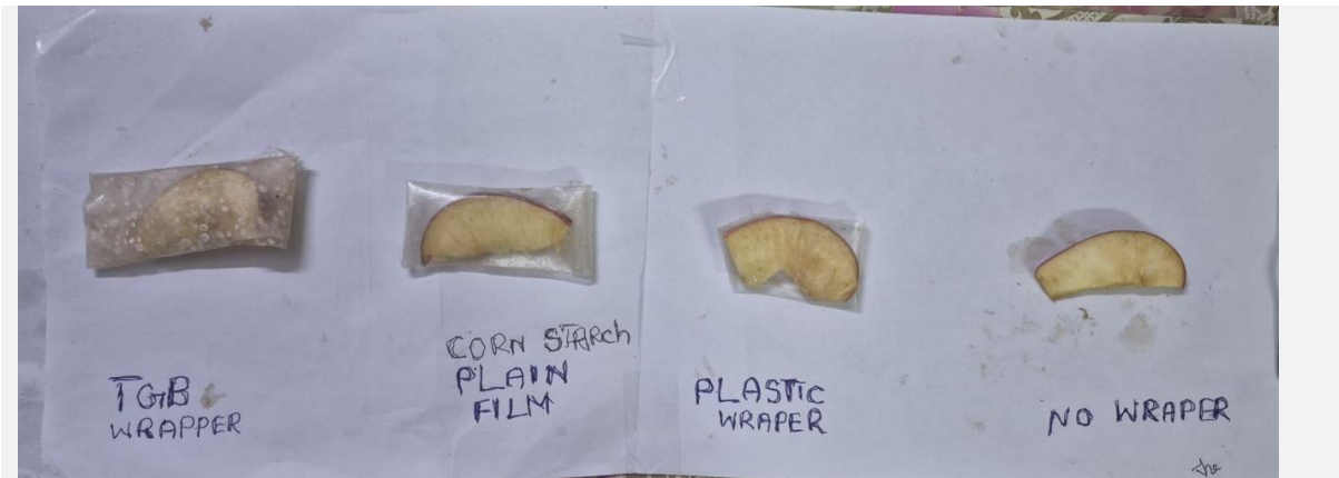
Fig. 6: Comparison of four apple samples wrapped with TGB film, plain starch film, plastic wrapper, and no wrapper for spoilage observation.
