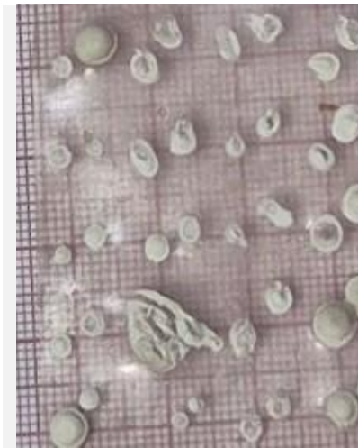
Fig.5(a ): Film with 2 dots/cm 2 – light pattern, clear surface
