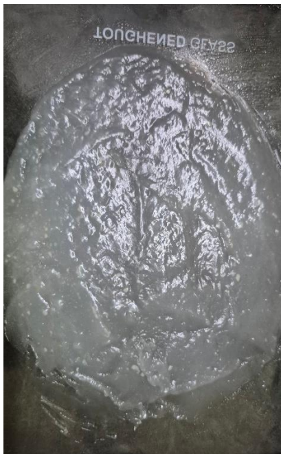
Fig. 3(g): Freshly poured film for drying.
