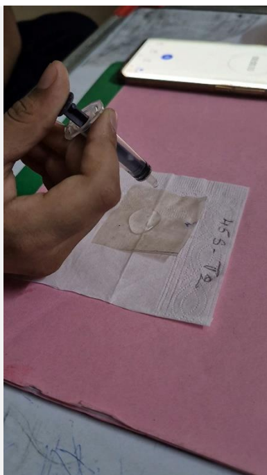
Fig. 4(d): Repeating the test for 45-second dip—film still intact, no visible wet spot
