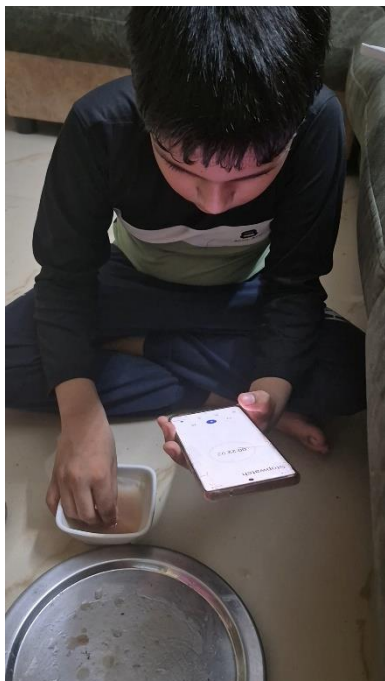
Fig. 4(a): Haris timing each dip duration (30 s, 45 s, 60 s) using a stopwatch during GSE film test.
